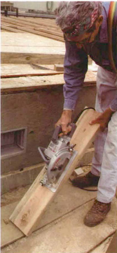
Flip the board for safe short rips. To rip short boards, plunge in about halfway down the board (above) and rip to the end. Flip the board and reinsert the blade into the kerf to finish the rip. Raise the board at the end of the cut to let the saw clear the material (right).
