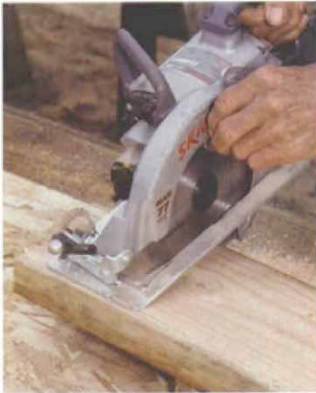
A 3-second crosscut. Make a plunge cut with your blade on the mark and the saw base square to the board (inset). With the saw running, lift the board so that the saw's weight helps to finish the cut (right).
